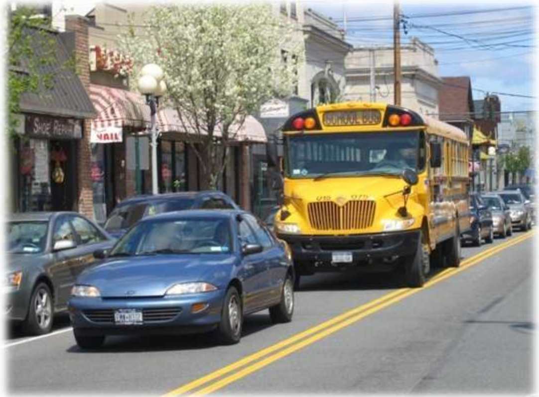
Narrow lanes along Main Street experience queuing when parallel parking maneuvers are executed; buses and trucks encroach on the centerline.
